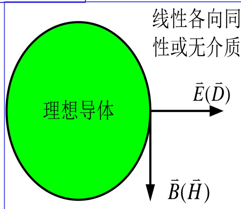
$$\text{边界条件} \left\{ \begin{array}{l} \hat{n} \cdot \vec{D}_2 = \rho_{sf} \\ \hat{n} \times \vec{E}_2 = 0 \\ \hat{n} \cdot \vec{B}_2 = 0 \\ \hat{n} \times \vec{H}_2 = \vec{J}_{sf} \end{array} \right.$$
