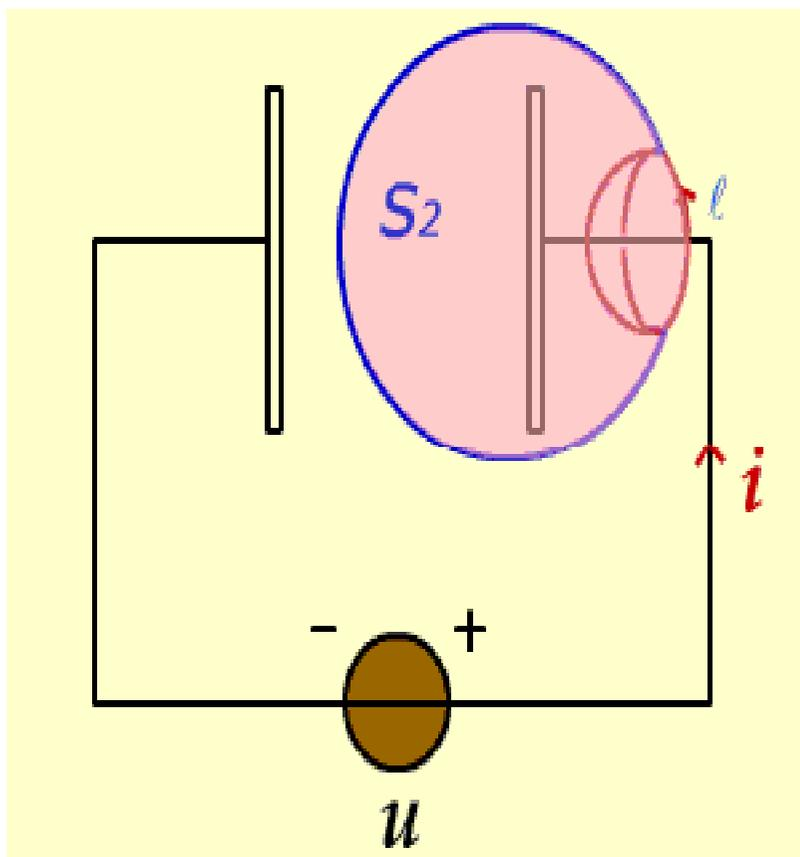
$$\left. \begin{aligned} \oint_l \vec{H} \cdot d\vec{l} &= \int_{S_1} \vec{J} \cdot d\vec{S} = i \\ \oint_l \vec{H} \cdot d\vec{l} &= \int_{S_2} \vec{J} \cdot d\vec{S} = 0 \end{aligned} \right\} \text{矛盾}$$
